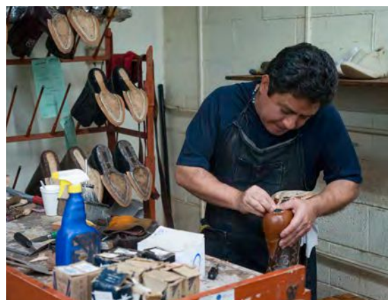
Boot maker Jose Pena nails a steel shank into a custom fitted cowboy boot at Little's Boot Company.
